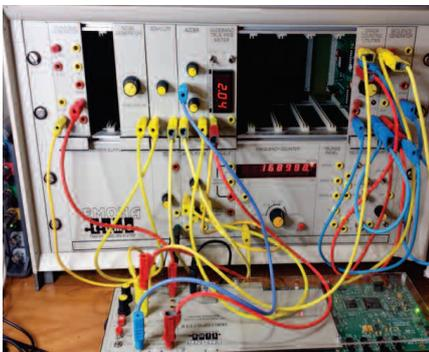
TIMS Turbo Coding experiment implementation with noisy baseband channel and BER measurement.
