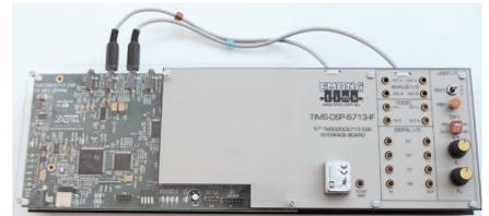
TIMS-DSP-6713 floating point DSP module used to implement the Turbo Coding algorithms.
